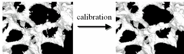
Figure 4: Calibration of the three dimensional CMT image
