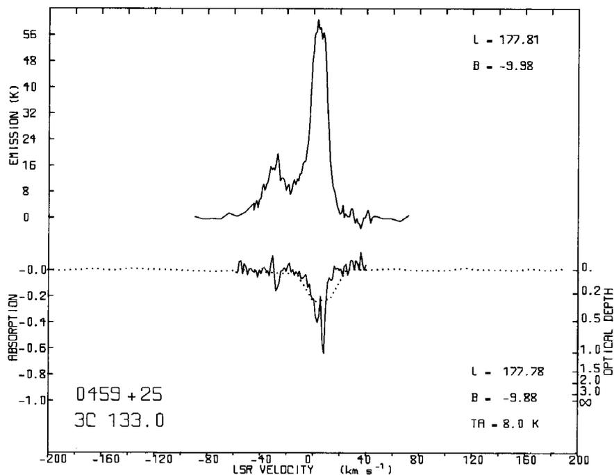
**Fig. 8.** H I 21-cm emission and absorption profiles towards 3C 133. Emission: spectrum in the region of 3C 133 from the Berkeley H I emission survey (Heiles and Habing, 1974). Absorption: spectrum from the Nançay H I absorption survey (Crovisier et al., 1977). The resolution is 60 kHz (dotted line) and 6 kHz (full line)
