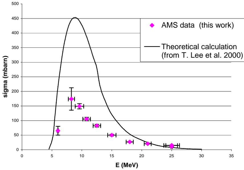
**Fig. 50: The excitation function of the  $^{24}\text{Mg}(^3\text{He,p})^{26}\text{Al}(5^+, t_{1/2}=0.716 \text{ Myrs})$  reaction deduced from AMS measurement (this work) compared to the theoretical calculation used in [2, 3].**
