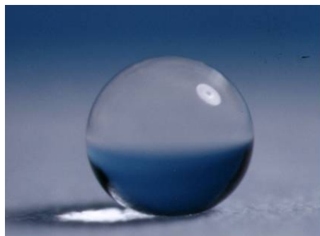
Figure 2.1: A drop of water on a super-hydrophobic (which doesn't like water) substrate adopts a spherical shape [1].
