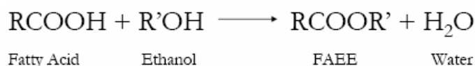
Figure C.1: Fatty Acid Ethyl Esters (FAEEs) are the esterification products of ethanol and fatty acids.
