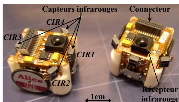
FIG. 8.4 – Mini-robots ALICE
