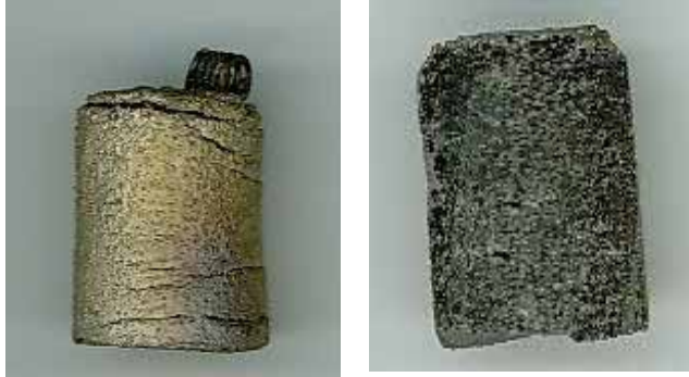
Figure 32: a) Surface of the reacted sample, Ti/80wt.% TiB, in the form of a layered pattern, b) Section of the sample, evidence of the internal porosity.
