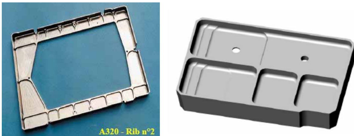
Figure 65: a) Rib of the engine pylon (A320), dimensions 600x400x80mm 4Kg, b) "first demonstrator" (simplified rib), dimensions 300x200x40mm, 12Kg.
