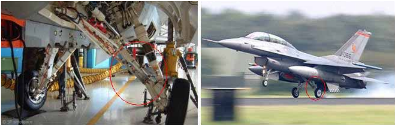
Figure 10: a) Installation of the TMC Lower Drag Brace in the F16 Main Landing Gear, b) Touchdown (SP Aerospace, 2003).
