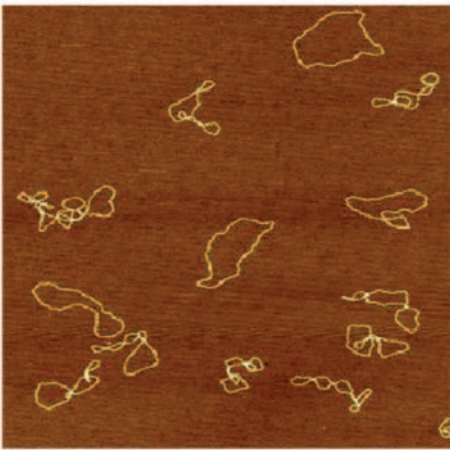
Figure 1. Mix of relaxed and supercoiled pTZ18R DNA plasmids adsorbed onto mica and imaged in air.
