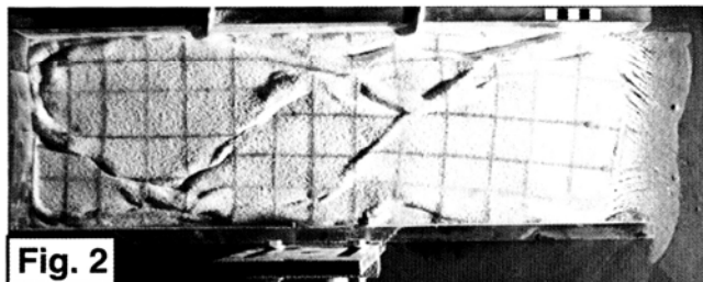
Fig. 2: Surface of 3-layer model (ductile upper mantle, ductile lower crust, brittle upper crust) after 50% shortening between parallel boundaries. Convergence direction was at 90° to the long side of the picture.
