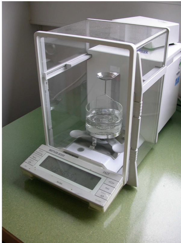
Figure 3.8: Picture of the balance used for the density measurements.
