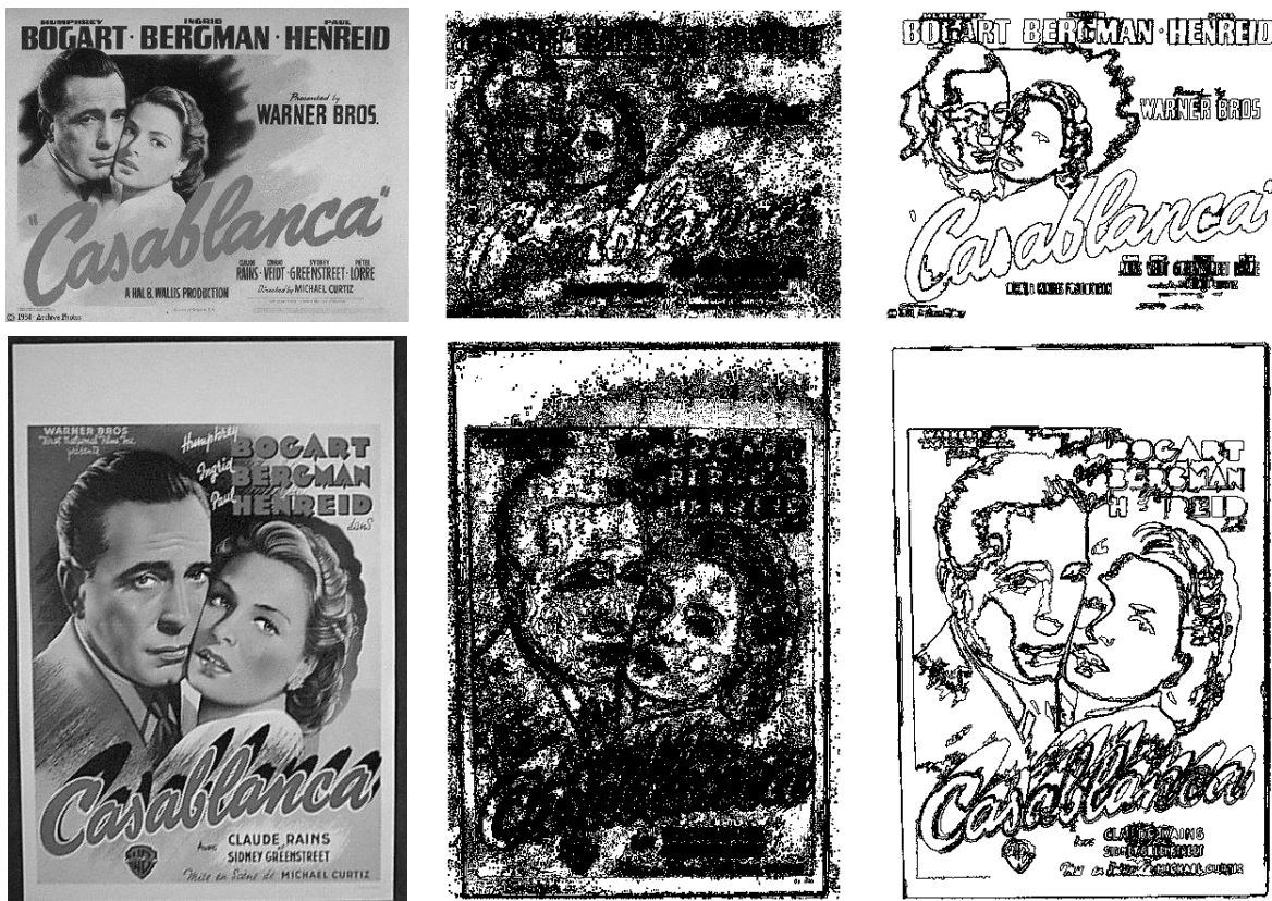
Figure 1.11: Two examples of level lines extraction. Left: original images. Middle: a subset of the level lines (quantization step for the gray levels is 20). Right: local meaningful level lines, obtained by the algorithm described in Chapter 4. The upper image will be referred as the “target image”. It generates 385 local meaningful level lines (among 359, 263). The lower image will be referred as the “database image”. This latest image generate 577 local meaningful level lines (among 462, 912). We aim at matching shapes in the target image with shapes in the database image. Looking closer to the images, we notice that the images show in fact dissimilarities: the actors’ faces are stylized in the database image whereas they correspond to a photography in the target image, the word “Casablanca” slightly differs, etc.
