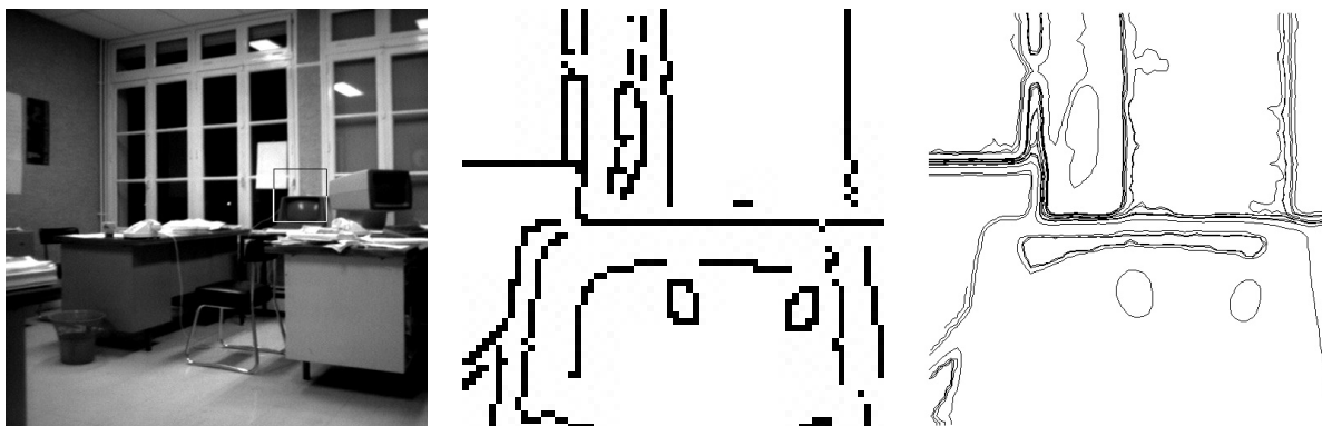
Figure 4.8: Junction and level lines. On the left, the original image. Middle, Haralick's detector implemented with Canny's filter on the area designated on the left image. Note how the contour is broken at the junction, due to the bad estimate of the gradient direction, and the high number of edge pieces. Right: detailed view of meaningful boundaries on the region. There are two level lines, each corresponding to an edge part.
