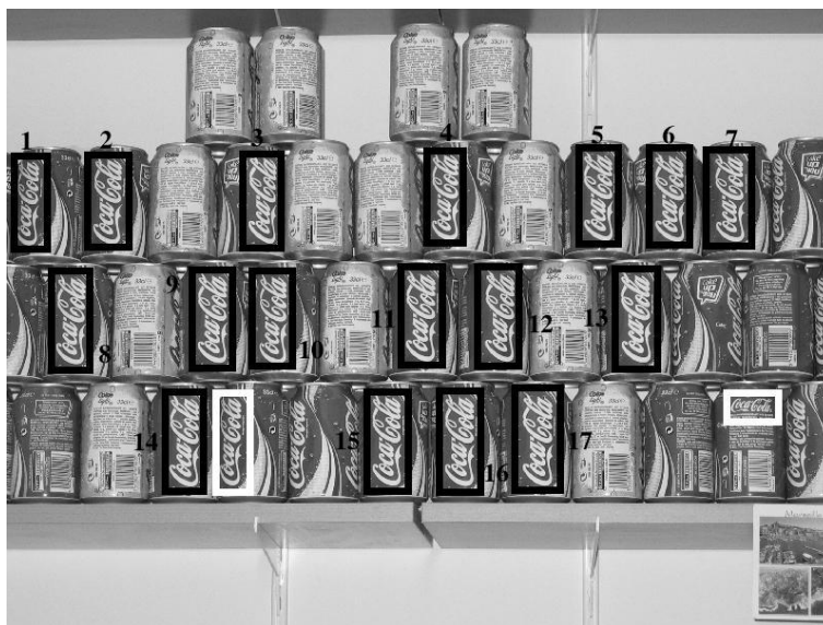
Figure 13.21: “Coca-Cola 2” experiment: maximal meaningful groups. 19 groups were detected as maximal meaningful groups. Among them, 17 correspond to groups in the black rectangles (see table 13.1 for their NFA_g ). In rectangle nb. 17 there is also a group due to strobe effect (Figure 13.23). The other maximal group is a casual detection (Figure 13.24). The misses shown in white rectangles are explained in Figure 13.22.
