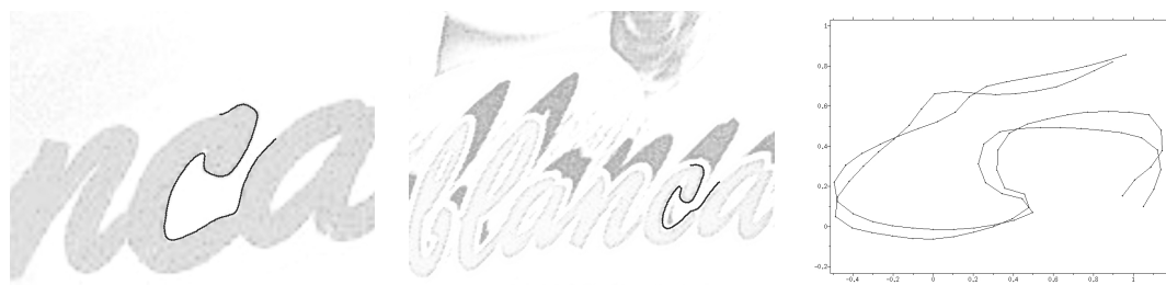
Figure 9.18: Casablanca experiment: match between shape elements which semantically correspond, but shows an NFA close to 1 ( NFA = 0.13 ). Notice however that the fonts of the characters are not the same, and that the shape element is not very discriminatory. This explains why the NFA is high.
