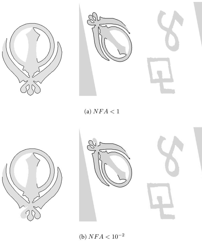
Figure 9.2: Affine invariant semi-local recognition: meaningful matches ( NFA < 1 ) between shape elements. No false match was detected.
