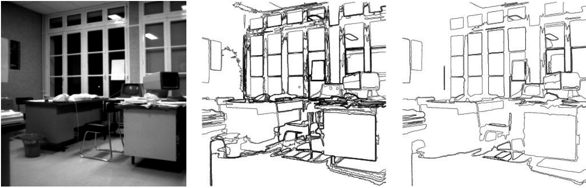
Figure 4.15: Regularity detectability. Left: original image. In middle, we display the 204 detected contrasted smooth boundaries as defined in Definition 4.5. On the right, the 96 smooth boundaries, with no contrast information, defined in (4.17). All the main boundaries are already present. Of course, contrast may be the main cause of small NFA, since regularity acts at larger scales. For instance, the window panes have NFA about 10^{-150} with contrast and 10^{-15} with regularity only (which still make them detectable in any image database). The desk on the bottom right has a NFA equal to 10^{-60} with contrast and 10^{-20} with regularity, which is already very small.
