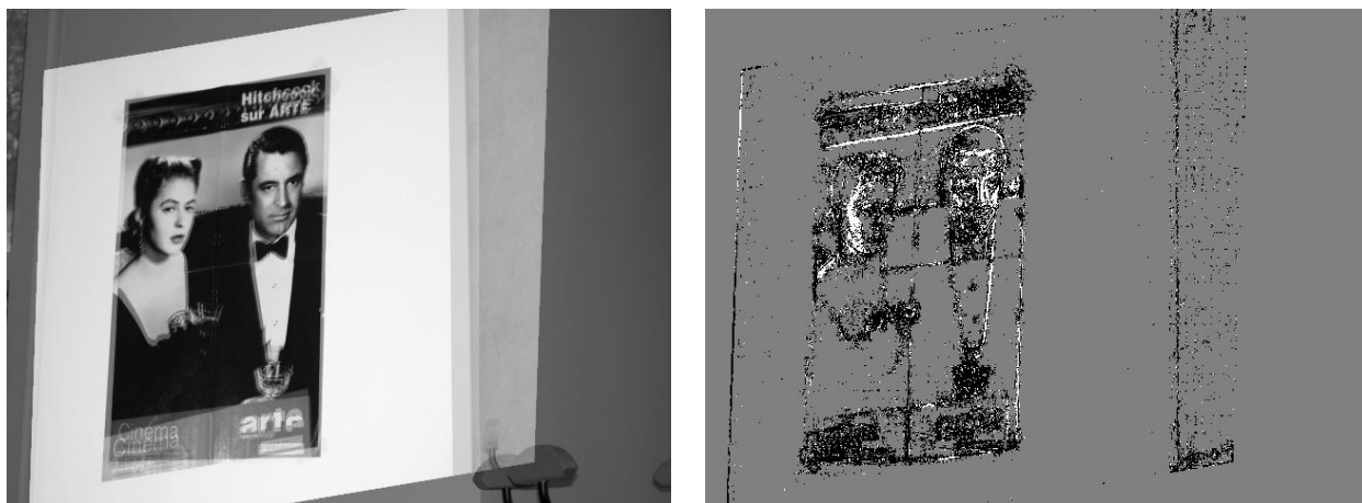
Figure 14.16: Hitchcock 2 experiment: all 16 meaningful matches were spatially coherent; the group made by all of them was detected as the only maximal meaningful group ( NFA_g = 1.4 \cdot 10^{-75} ). Left: registration of the target image and superimposition on the scene image. Right: gradient orientation comparison.
