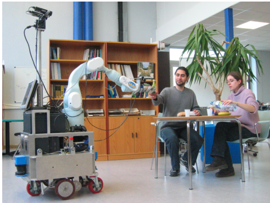
Figure 1 – Hand over task, the planner generates two grasps, one is executed by the robot and the second one tells us that at least the object is graspable, even if we cannot assure that the human will find the same grasp.
