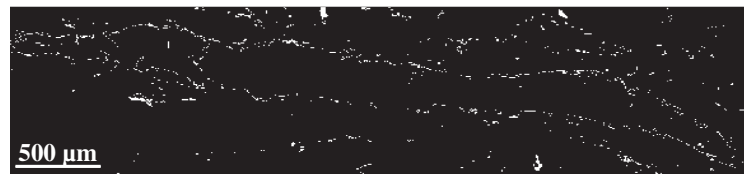
Fig. 6. Image of chlorite analyses that were discarded (white pixels) or accepted (black pixels) on the basis of stoichiometric constraints. The discarded pixels correspond to contaminated analyses, e.g. by mica on the limit of the crystallization tail, or iron oxide.
