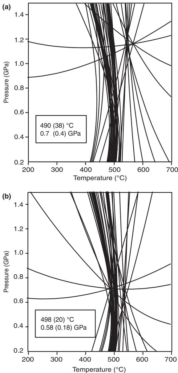
**Fig. 9.** Multiequilibrium calculation for Chl-Gt-Qtz-H<sub>2</sub>O assemblages with two different high temperature chlorite compositions corresponding to the 440–460 °C (a) and 480–520 °C (b) groups in Fig. 5b. The average *P*–*T* values and the standard deviations (in parenthesis) are indicated on the figures. The compositions used for the calculation are listed in Table 1.
