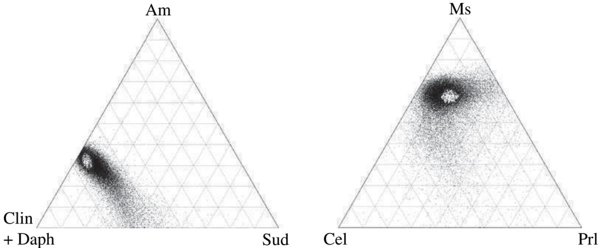
**Fig. 9.** Plot of the phyllosilicate compositions from the Sambagawa sample in Amesite-(clinocllore + daphnite)-sudoite (a: chlorite) and celadonite-muscovite-pyrophyllite (b: phengite) end-member ternaries. Each black point represents the composition of one pixel. White points are 1000 chlorite and phengite analyses calculated by the Monte Carlo method. The analytical uncertainties calculated from the Monte Carlo simulation are given in Table 1.
