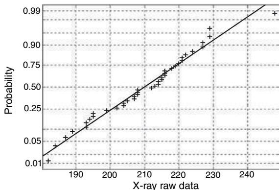
**Fig. 2.** Poisson probability plot of theoretical probability values as a function of measured raw values for a same pixel during time. Data are well fitted by a line (consistent with the Poisson counting statistic) that can be used to derive the law parameter.
