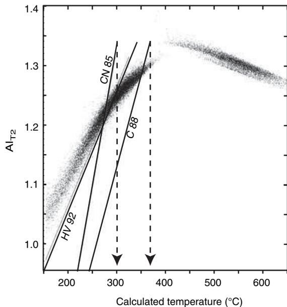
**Fig. 6.** Plot of calculated (0.5 GPa) temperature of chlorite ( $\text{Fe}^{3+}$  minimum = 0) occurring in Fig. 2 v. tetrahedral aluminium content. For comparison, the temperatures calculated from the empirical thermometers from Cathelineau & Nieva (1985) (CN 85), Cathelineau (1988) (C 88) and Hillier & Velde (1992) (HV 92) are also shown (straight lines). The maximum temperatures predicted by these geothermometers are shown by the dashed arrows (300–360 °C).
