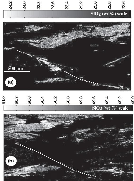
**Fig. 8.** Maps of SiO<sub>2</sub> content (in wt%) in chlorite (a) and phengite (b) from the Spitzbergen sample. The dashed line shows the location of the shear zone.
