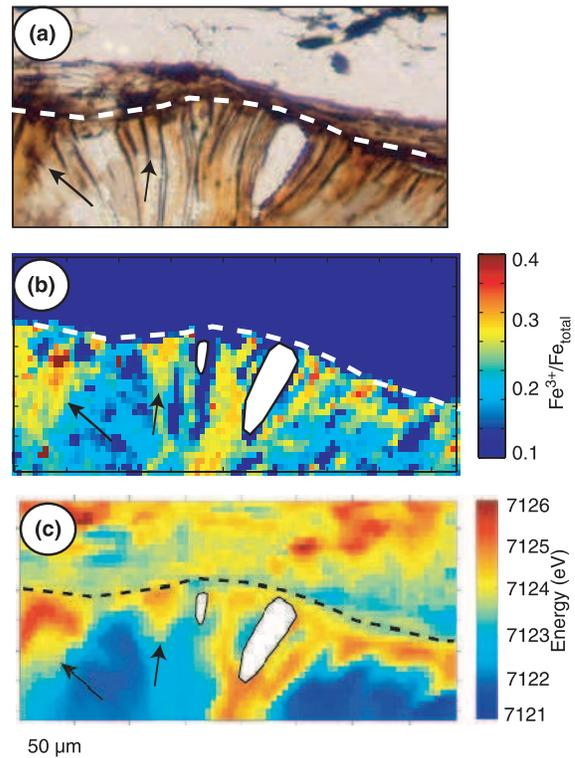
**Fig. 3.** Comparison of (a) optical microscope image of the zone A in Fig. 2b with calculated  $\text{Fe}^{3+}/\text{Fe}_{\text{total}}$  map (b) and map of iron K-edge energy derived from arctangent fits of the XANES spectra (c). The dashed line shows the outer border of the chlorite crystallization tail.
