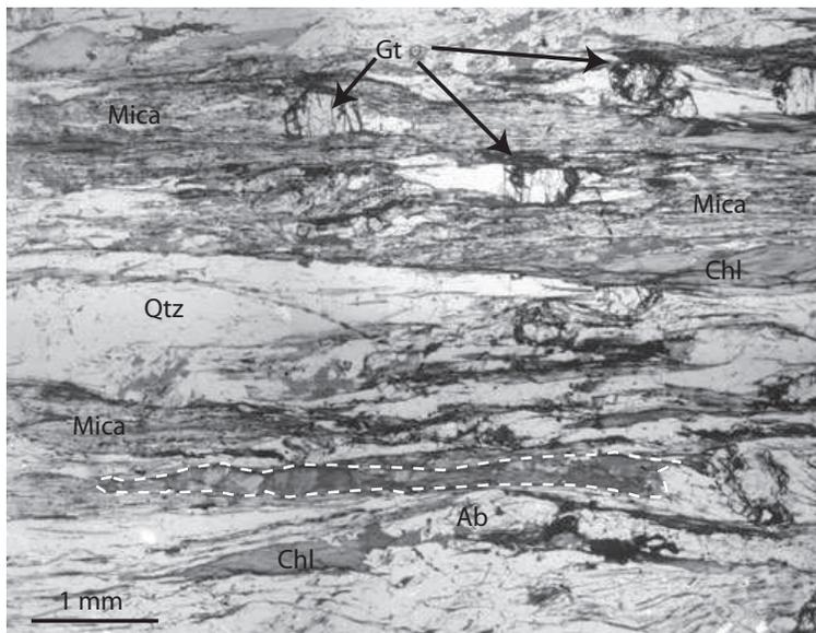
**Fig. 1.** Optical microscope image of the studied zone of the studied thin section. The dashed line indicates the chlorite crystallization tail shown in Figs 2–4. Chl, chlorite; Ab, albite; Qtz, quartz; Grt, garnet.
