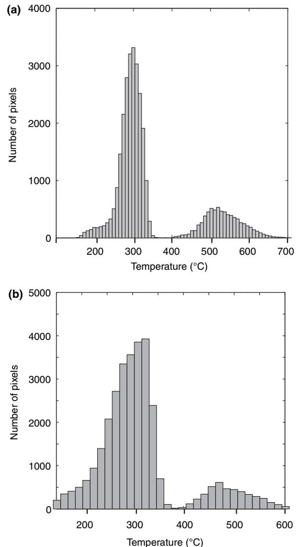
**Fig. 5.** Distribution of pixels as a function of temperature calculated at 0.5 GPa for the chlorite occurring in Fig. 2. The temperatures were calculated in panel a assuming a minimum amount of  $\text{Fe}^{3+}$  in chlorite. In panel b, the high temperatures obtained in panel a (above  $475^\circ\text{C}$ ) were recalculated by assuming  $\text{Fe}^{3+} = 0.05 \times \text{Fe}_{\text{total}}$ .
