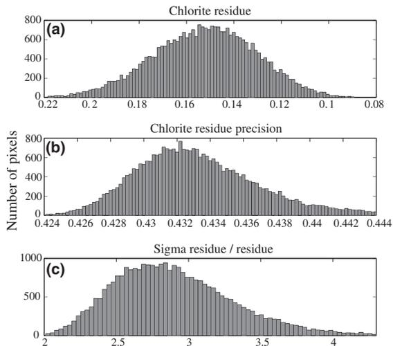
**Fig. 5.** (a) Histogram of the chlorite residue obtained for the Sambagawa sample. The shift from zero of the histogram centre is indicative of systematic analytical and/or calibration errors. (b) Histogram of the residue precision. (c) Histogram of the ratio between residue precision and residue values.
