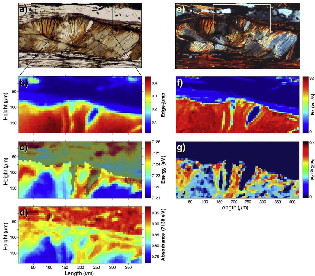
**Figure 3.** Rock sample mapping: (a) polarized optical image (chlorite in the middle, quartz at the top, and phengite between chlorite and quartz and at the bottom); (b) iron content (edge-jump); (c) iron redox (edge-position); (d) iron speciation (absorbance contrast at 7137 eV); (e) crossed-polarizer optical image; (f) quantitative iron content map (from electron microprobe analyses); and (g) quantitative iron redox map (from thermodynamics).
