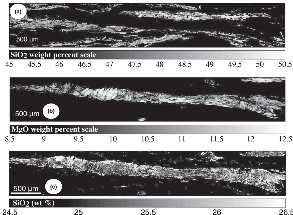
Fig. 7. Maps of mineral composition (in wt%) from the Sambagawa sample. (a): SiO<sub>2</sub> in phengite, (b) and (c): MgO and SiO<sub>2</sub> in chlorite.
