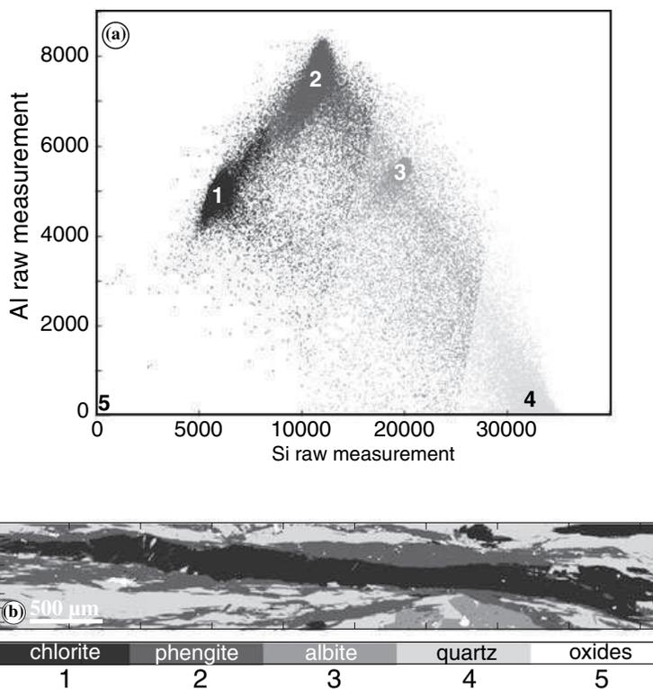
**Fig. 4.** (a) Projection of all raw pixel analyses of the Sambagawa sample on a Si v. Al plane. (b) Representation of the masks created with the statistical cluster analysis ‘K-means’ of Matlab<sup>®</sup>.
