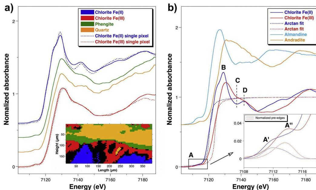
**Figure 4.** (a) Averaged and “single-pixel” XANES spectra based on the different masks of the maps. Blue, chlorite-Fe(II); green, phengite; orange, quartz; and red, chlorite-Fe(III). (b) XANES spectra for chlorite-Fe(II) and chlorite-Fe(III) with the arctangent fits (dashed lines) and a zoom on the pre-edges showing also their normalization (dashed lines). XANES spectra of almandine and andradite are shown to illustrate of the  $K$ -edge shift of reference compounds.
