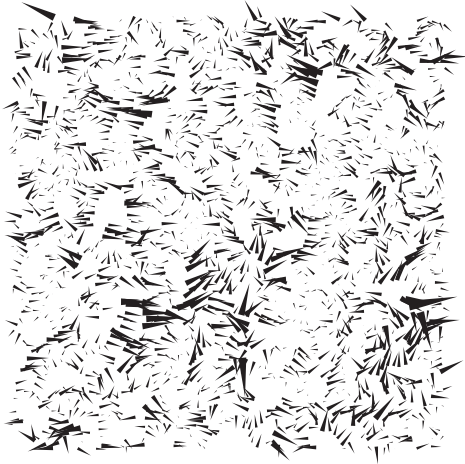
FIG. 1. Inhomogeneous part \delta u(\mathbf{r}) of the displacement field \mathbf{u}(\mathbf{r}) for the imposed macroscopic uniaxial strain in elongation \epsilon_{xx} = 5 \times 10^{-3} for a silica glass containing N = 42\,000 particles ( L = 83.8 Å). Projection of the field is done on the (x-z) plane for all particles with position \mathbf{r} close to the plane. The arrow length is proportional to \delta u(\mathbf{r}) and scaled by a factor of 150. The field resides in the linear elastic regime, i.e., has a magnitude varying linearly and reversibly with the applied deformation. As visual inspection shows, it is strongly spatially correlated and involves a substantial fraction of all atoms.
