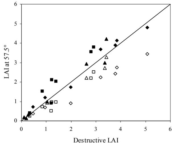
Figure 11 : On this graph, the destructive ( $LAI_{dest}$ ) LAI value was compared to the Lang and Xiang ( $LAI_{LX}$ , black symbols) and effective ( $LAI_{eff}$ , open symbols) LAI values estimated gap fractions at  $57.5^\circ$ . The 2004 and 2005 data are plotted.
