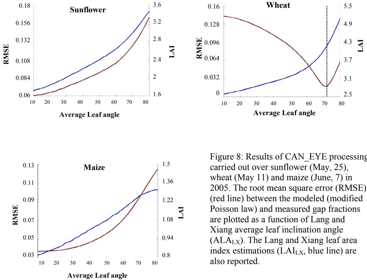
Figure 8: Results of CAN\_EYE processing carried out over sunflower (May, 25), wheat (May 11) and maize (June, 7) in 2005. The root mean square error (RMSE) (red line) between the modeled (modified Poisson law) and measured gap fractions are plotted as a function of Lang and Xiang average leaf inclination angle ( $ALA_{LX}$ ). The Lang and Xiang leaf area index estimations ( $LAI_{LX}$ , blue line) are also reported.
