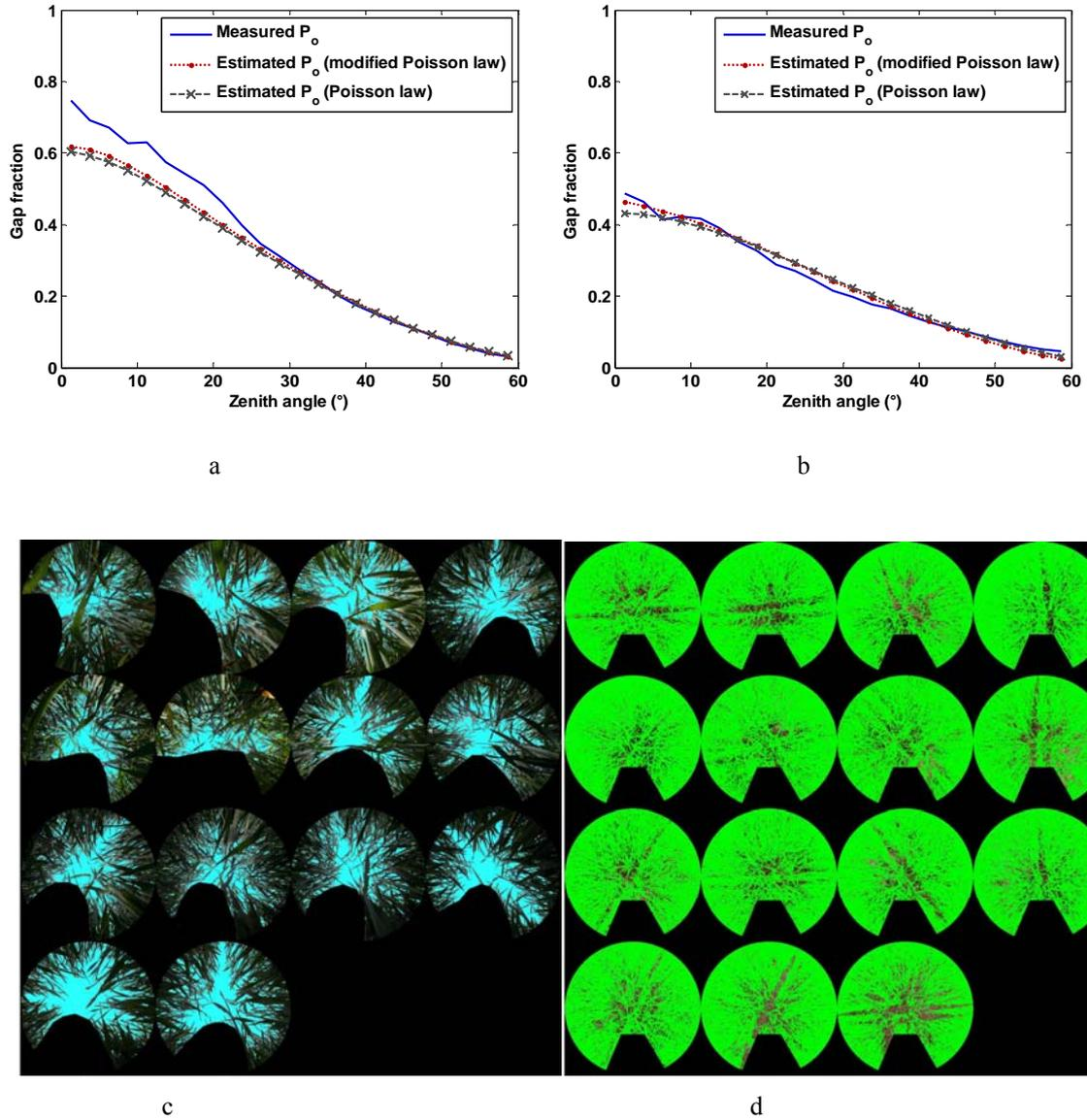
Figure 3 : Gap fraction ( $P_0$ ) measured on wheat on May 11, 2005 . (a) with upward photographs (b) with downward photographs. (c) Upward CAN\_EYE classification (only sky have been classified) and (d) downward CAN\_EYE classification (only vegetation have been classified).
