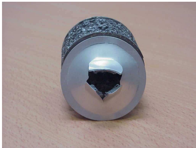
FIGURE 3.20: Post-perforation de la plaque secondaire.
