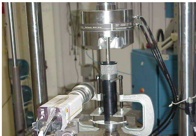
FIGURE 3.18: Montage quasi-statique de perforation.
