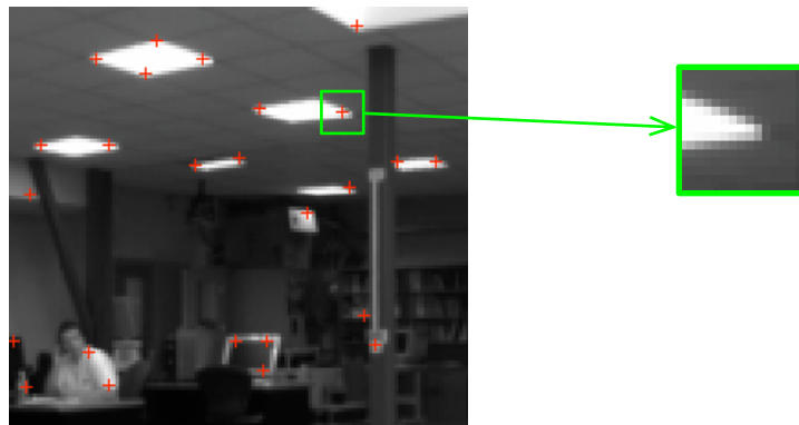
Figure 2.14: Feature detection ( red ) and patch definition ( green ).
