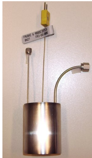
Figure 13: Cellule type blowdown
