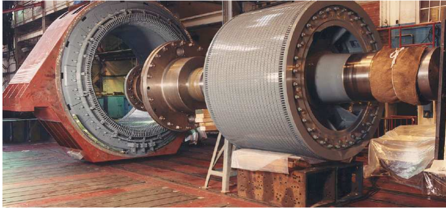
Figure 1.12 : Machine asynchrone de 4.7 MW, 45tr/mn [30]
