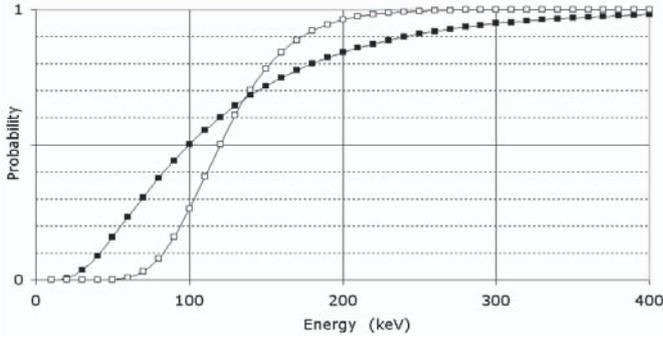
**Fig. 10.** For PMT<sub>1</sub>(solid),  $E_{th} = 100$  keV and  $a = \sqrt{50}$ , for PMT<sub>2</sub>(open), 120 keV and  $\sqrt{10}$ . These curves illustrate the large differences between ACS crystals and PMTs combinations.
