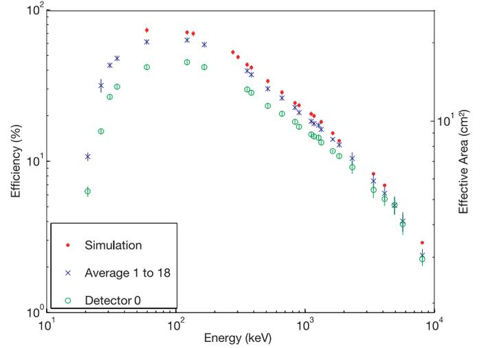
**Fig. 2.** Full-energy peak efficiency for sources on the SPI optical axis ( $\alpha = 0^\circ$ ), without mask. An average for detectors 1 to 18 is shown; detector 0 is plotted separately (see Sect. 5.2). The measurements are compared to Monte-Carlo simulations.
