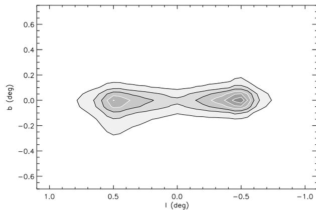
**Fig. 9.** Maximum entropy image in the 1173 keV  $^{60}\text{Co}$  line shows the capability of the instrument to separate sources closer than the angular resolution, where the signal-to-noise ratio is good. The sources are separated by  $1^\circ$ .
