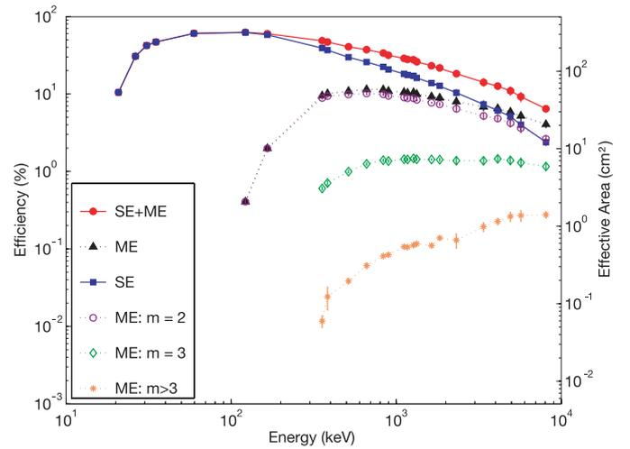
**Fig. 4.** Full-energy peak efficiency for SE, ME and all events (SE+ME) and for ME with multiplicity  $m = 2, 3$  and  $>3$ , for the camera without mask. The effective area is the geometric area multiplied by the efficiency.
