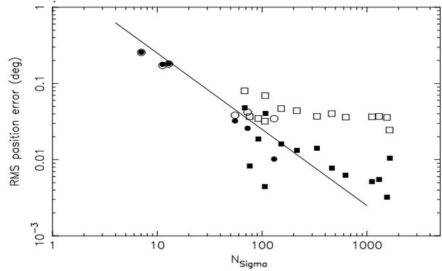
**Fig. 8.** The error in the determination of a narrow line source position from analysis of calibration data. Squares: subsets of data, circles: mean of 10–20 trials with samples of random noise added. Open symbols: deviations from the nominal position, filled symbols: deviations from an assumed displaced source position. The line corresponds to  $2.5^\circ/N_\sigma$ .
