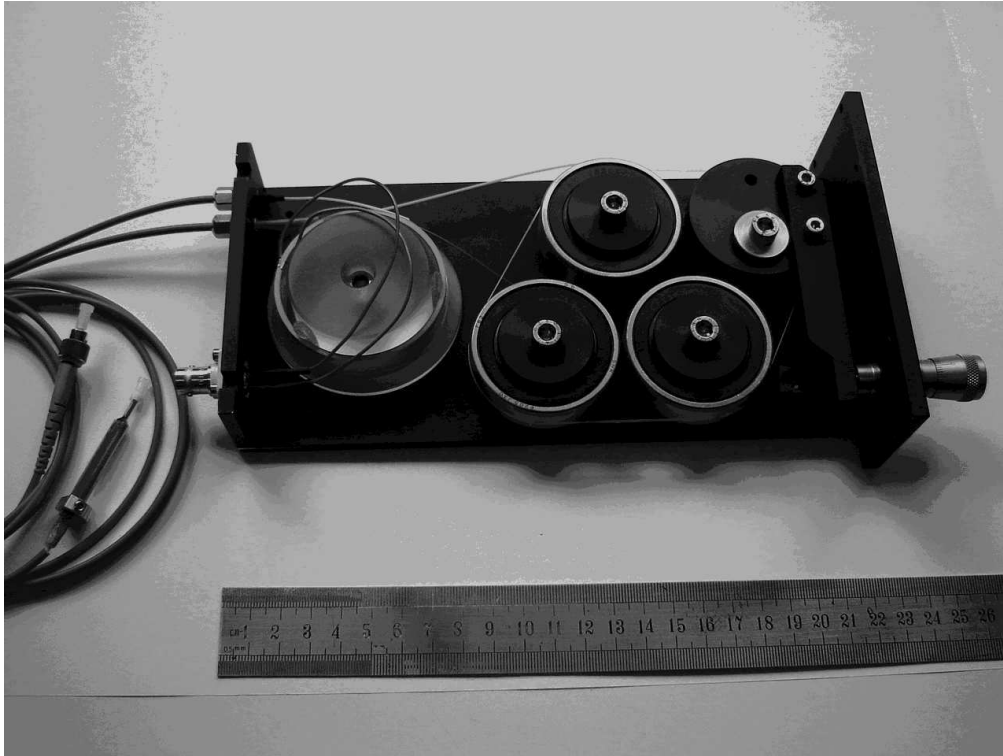
Figure 4. Fibered delay-line and piezo-electric cophasing system, from the XLIM laboratory. Both are integrated in the same box.
