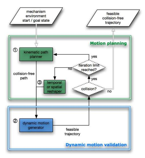
**Figure 5.1:** Our three-step approach consists in (1) finding a kinematic path for the mechanism, (2) generate, with available dynamic controllers the required motions to execute this path, and (3) reshape the trajectory to eliminate the collisions appeared due to the dynamic behavior of the system.
