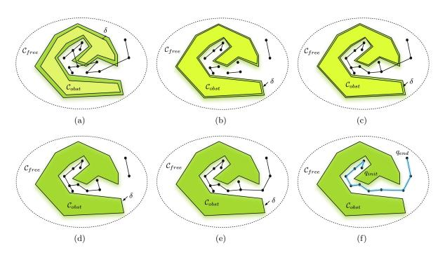
Figure 2.4: (a) A first tree is grown allowing a large value of dynamic penetration  $\delta$ . (b) Decreasing the value of  $\delta$  local paths are tested for collision and removed if collision is found. (c) A new tree is grown using the remaining roadmaps and the decreased value of allowed  $\delta$ . (d) and (e) The process is iteratively performed until the tree is entirely in  $\mathcal{C}_{free}$ . (f) A collision-free path is found in the remaining tree from  $q_{init}$  to  $q_{end}$ .
