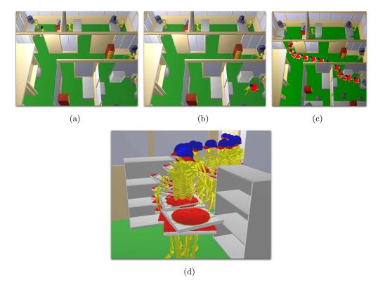
**Figure 4.12:** (a) Initial configuration. (b) Final configuration. (c) Some configurations of the computed trajectory. (d) The mannequin moves his elbow in order to avoid collision with the bookshelf.
