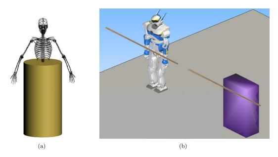
**Figure 3.6:** For obtaining a first trajectory for the system, a reduced model that bounds the robot's locomotion DOFs is used. (a) Our virtual mannequin, Eugène, inside its bounding box. (b) HRP-2 is reduced to a box that navigates in the environment with an object attached to it.
