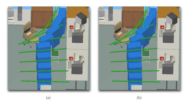
**Figure 6.4:** Two kinematic paths computed for the simplified model of the system and with two different clearance parameters. The difference can be seen in the configurations near the cabinet.
