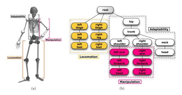
**Figure 3.4:** (a) The system's DOFs are decomposed in three groups: locomotion, manipulation and adaptability. (b) Tree-like structure of a humanoid character and its functional decomposition. The edges represent the joints of the articulated figure and the nodes represent the rigid-bodies that link them.
