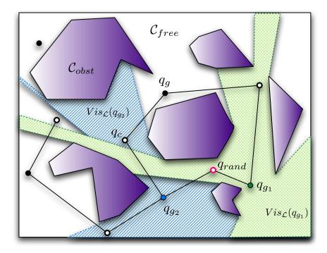
**Figure 2.3:** The Visibility-PRM algorithm produces a compact roadmap around obstacles with only a few nodes:  $guards \ q_g$  (dark circles) and  $connectors \ q_c$  (in white). A new randomly drawn configuration  $q_{rand}$  is added as a guard if it covers a previously unseen visibility domain with a given  $\mathcal{L}$  or as a connector if it serves as liaison between at least two connected components.
