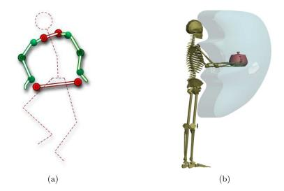
**Figure 4.3:** (a) The closed kinematic chain formed when grasping an object with two hands is decomposed in active (the object and the clavicles) and passive (the arms) parts in order to plan its motion. (b) An approximation of the space that can be reached by a character holding an object with two hands.
