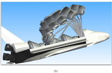
**Figure 5.6:** Swept volume throughout the collision-free dynamic trajectory. The collisions found after simulating the dynamic behavior were corrected with the temporal reshaping algorithm.
