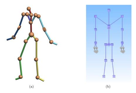
**Figure 3.2:** Hierarchical tree-like structure of a humanoid mechanism with a 6-DOF root placed on the waist. (a) A human-like virtual character is modeled with 18 joints and 50 rotational DOFs. (b) The HRP-2 humanoid robot skeleton has, as the human character, five kinematic chains. It is composed of 31 rigid bodies connected with 30 revolute joints.
