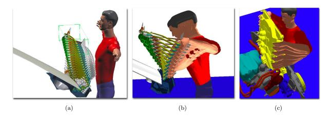
**Figure 4.2:** (a) Windscreen wiper motor assembly. A first collision-free path is computed for the part alone. (b) The character follows the path using an inverse kinematics operator to grasp the object. (c) A radiator assembly with two-hand grasping.
