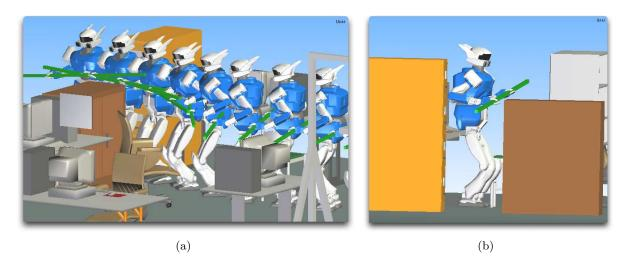
**Figure 6.7:** The dynamic trajectory is reshaped so as to avoid new collisions. The movement of the handled object drives the arms of the humanoid robot.
