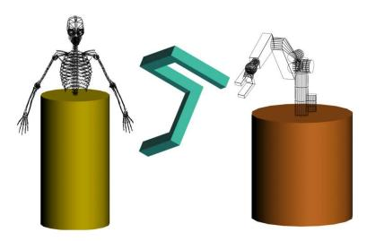
**Figure 4.6:** A 12-DOF reduced geometric model of the system is employed in the planning phase. Each of the bodies will have an associated steering method while planning a path for the system.
