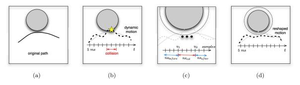
**Figure 6.6:** (a) Collision-free kinematic path. (b) Each configuration of the dynamic trajectory sampled at 5ms is checked for collisions. Colliding portions of the motion are identified. (c) A collision-free configuration for the upper body is found for each of the colliding ones by augmenting the minimum clearance value to the obstacle. (d) The new collision-free motion replaces the colliding one and smoothly interpolated with the rest of the trajectory.
