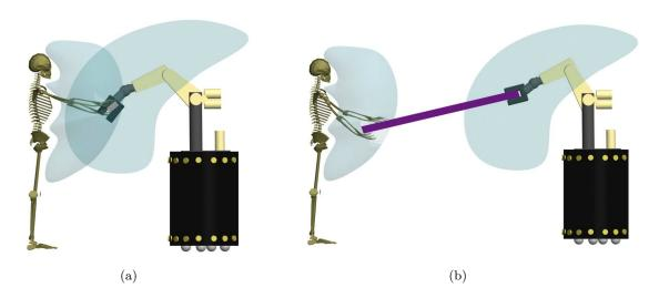
**Figure 3.5:** (a) Individual reachable spaces are intersected to obtain the cooperative reachable workspace, where the object is constrained to remain. (b) When manipulating a large object, the individual workspaces are enlarged by the objects size to compute the cooperative reachable workspace.
