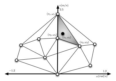
**Figure 4.4:** From Pettré and Laumond [2006]. Each captured locomotion cycle is represented as a point in the  $v - \omega$  space according to their average linear and angular velocity. A new walking cycle is obtained by from the interpolation of the three closest sources to the control input  $u(v, \omega)$ .
