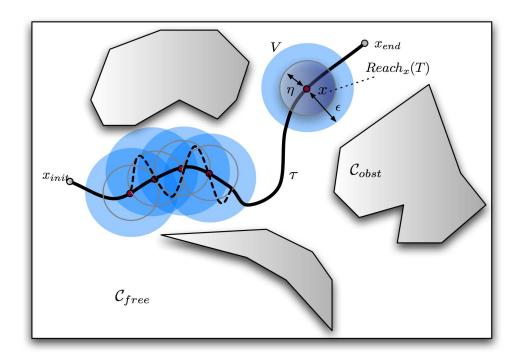
**Figure 2.6:** A system is small-time controllable from x if  $Reach_x(T)$  contains a neighborhood of x for all neighborhoods V for any time T > 0. If this is so, the system can be approximated to any  $\tau$  by a set of feasible maneuvers.
