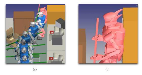
**Figure 6.5:** The path resulting from the kinematic motion planner is approximated with a dynamic walking pattern generator. (a) The dynamics of the task produces a deformation of the initially planned motion. (b) A collision is produced due to the weight of the bar, neglected during the computation of the first path.
