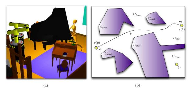
Figure 2.1: (a) Our version of the Piano Mover's Problem. Two robots and a virtual character cooperate to transport a piano in a workspace  $W \subset \mathbb{R}^3$ . (b) The configuration space is divided in  $C_{free}$  (light areas) and  $C_{obst}$  (dark areas). A path can be found between  $q_1$  and  $q_2$  because they lie in the same connected component of  $C_{free}$ , which is not the case for  $q_3$ .
