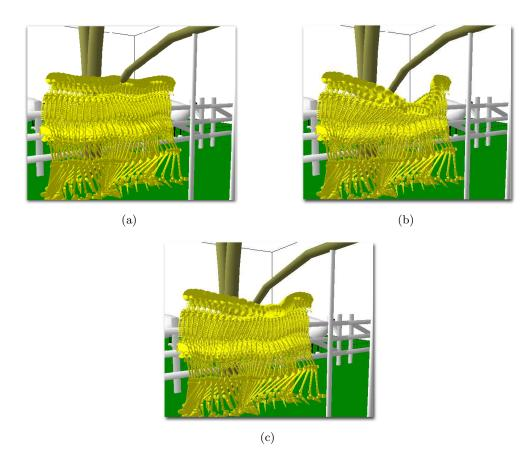
**Figure 4.9:** From Pettré [2003]. (a) After synthesizing locomotion, a collision is found in the mannequin's head with the tree branch. (b) The collision is solved by finding a random collision-free configuration within the joint limits and warped with the previous animation. (c) The solution is optimized to obtain a smooth motion.
