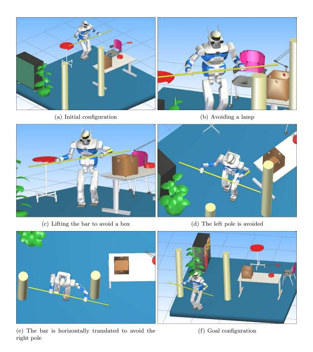
Figure 6.9: Simulation resulting from our 3-dimensional motion planner
