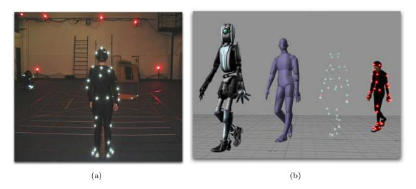
**Figure 4.1:** (a) VICON optical motion system in Paris. The performer wears reflective markers on his clothes (white spots). Position and orientation of the markers are recorded by 24 cameras (red spots) placed on the walls. (b) The recorded marker's information is processed to reconstruct the motion so it can then be fitted to a virtual skeleton.
