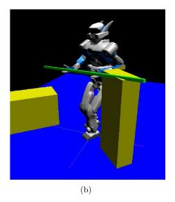
**Figure 6.2:** Simulation of the manipulation task we tackle in this work. Assigning a different weight to the bar leads to a different posture of the humanoid. (a) Light bar, no collision occurs. (b) Heavy bar, the bar collides with the obstacle.
