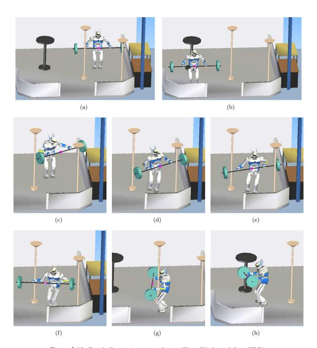
$\textbf{Figure 6.11:} \ \, \text{Dumbell experiment simulation (KineoWorks and OpenHRP)}$
