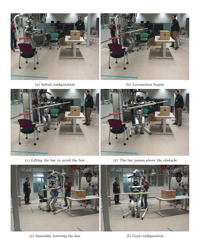
Figure 6.10: Real execution of a planned bar-carrying task
