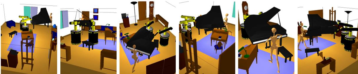
**Figure 4.17:** Two mobile manipulators and a virtual mannequin cooperating to transport a piano.
