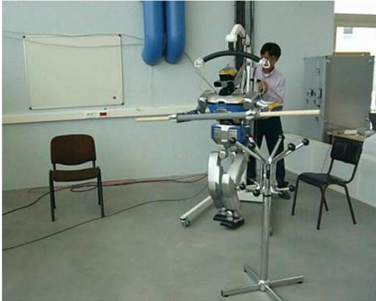
**Figure 6.1:** Humanoid platform HRP2-14 at LAAS-CNRS. In this work we consider the task of carrying a large object in cluttered environments.
