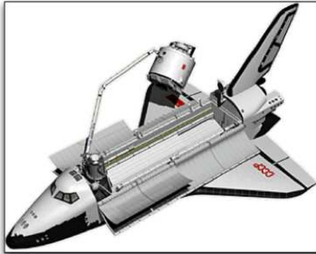
**Figure 5.2:** The Buran space shuttle has, in its middle part, a payload bay where the 6-DOF, 15.5m large RMS is installed (photo taken from <http://www.buran-energia.com>).
