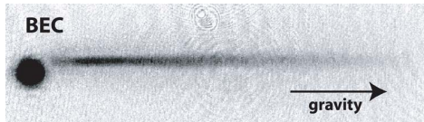
FIG. 12. 10 ms of atom laser. The BEC is displaced from the beginning of the beam due to a slight Stern-Gerlach effect at the switch off of the trap. The continuity of the laser beam shows qualitatively that the magnetic field is stable.
