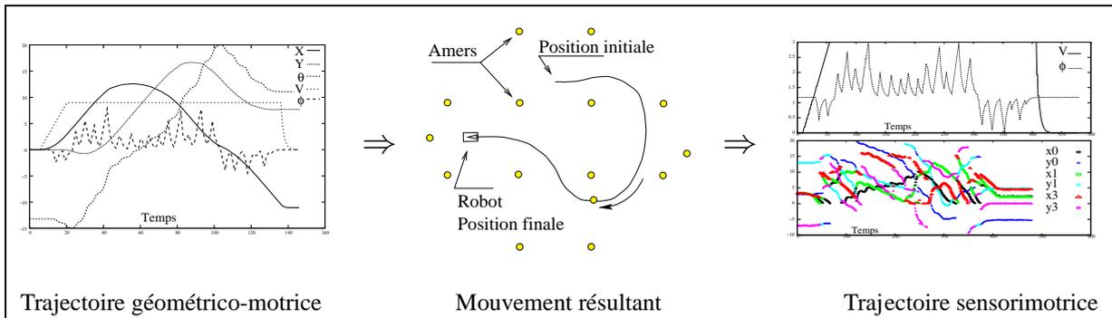
FIG. 3.2: Planification sensorimotrice.
