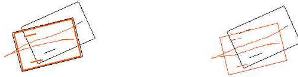
Figure III.6: Left: Elementary path with a cusp point as proposed in Figure III.4; Right: The corresponding path when the cusp point is computed as shown in Figure III.5
