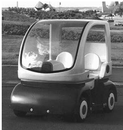
Figure V.1: The INRIA Rhône-Alpes' Cycab robot.
