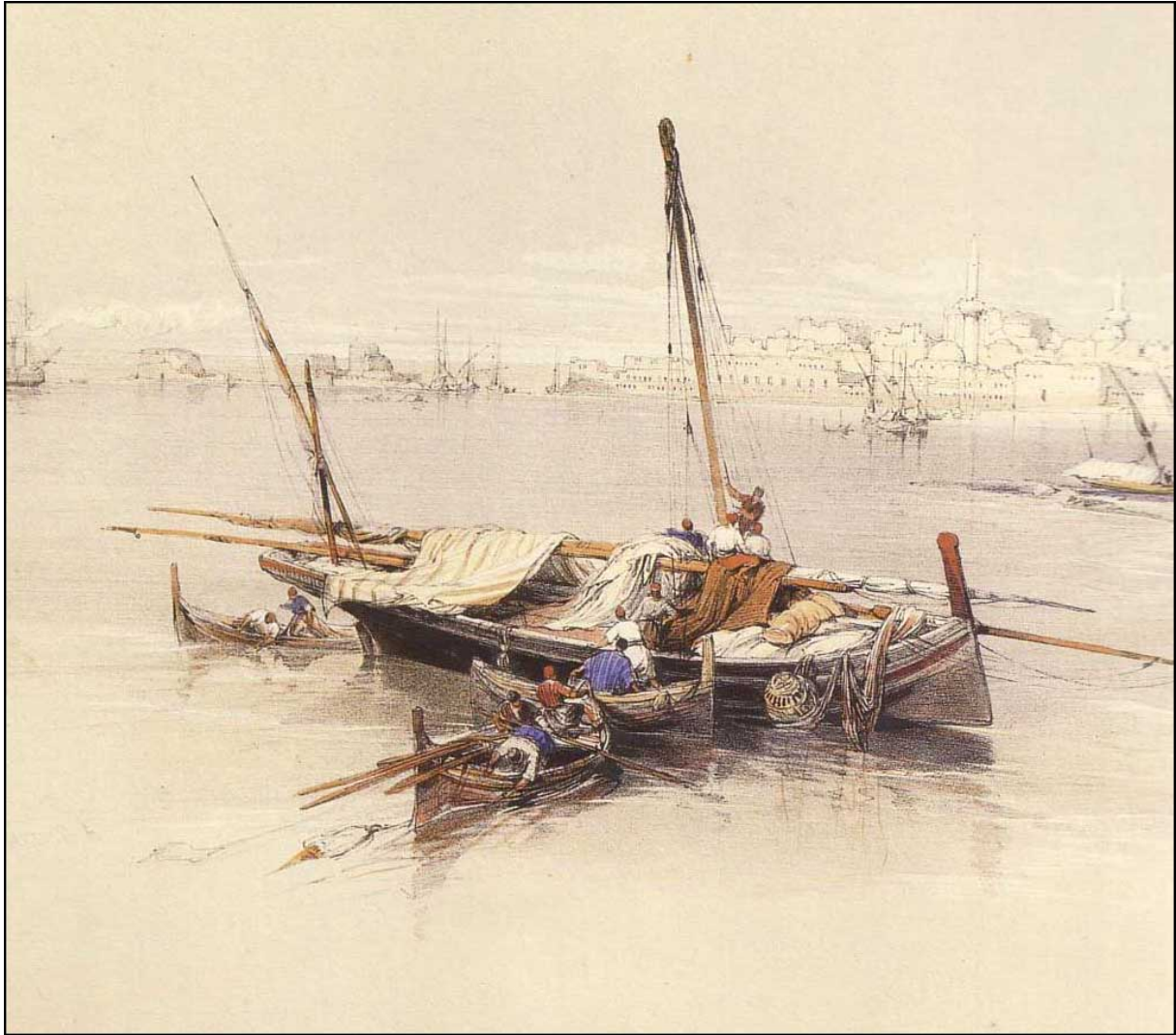
Figure 3.52: Nineteenth century lithograph engraving of lighter vessels being used to unload a sailing craft offshore at Acre in Palestine. The technique has probably evolved very little since the Bronze Age. The use of outer harbours in tandem with lighters greatly increased Tyre's capacity to receive and transit trade goods (full title of lithograph: Saint Jean d'Acre, from the sea , in David Roberts The Holy Land , 1842).
