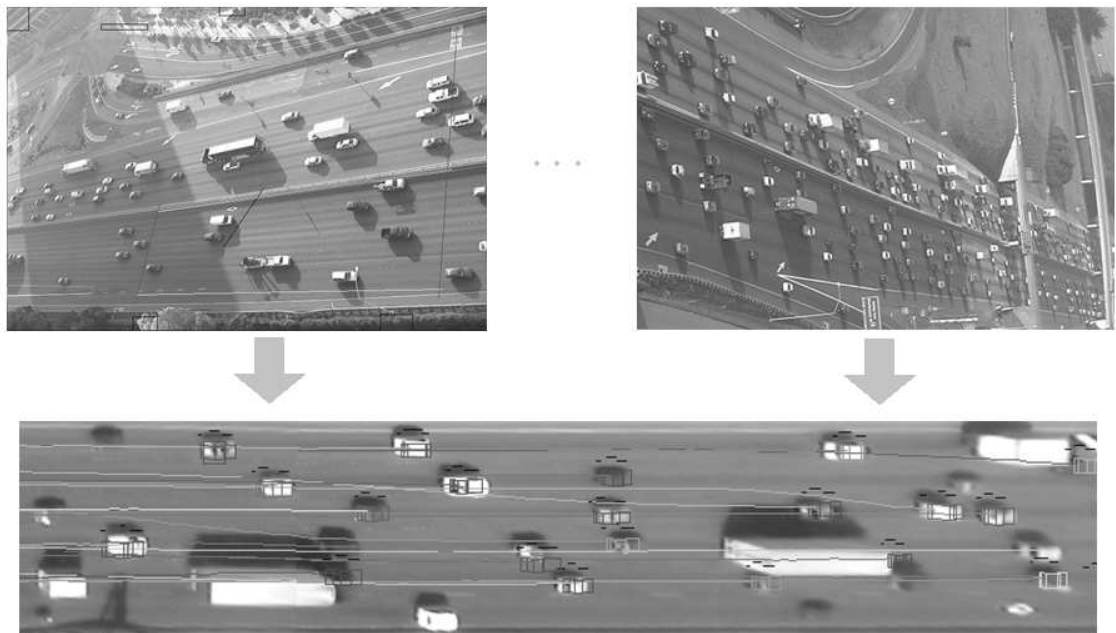
Figure 8.13: Two video frames and the reconstituted traffic picture (courtesy of FHWA).
