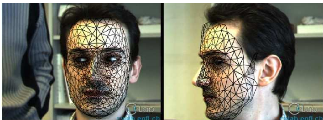
Figure 2.10: Vacchetti et al.'s grid based face tracker. The system requires a very high resolution face image to work [147]
