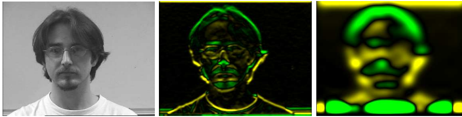
Figure 6.2: Example of receptive fields response to the first gaussian derivative G_{y,\sigma} at different scales \sigma . The left image is the original image. The middle image is the reponse to the derivative with \sigma = 2 pixels. The right image is the reponse to the derivative with \sigma = 10 pixels. Positive values are represented in yellow, negative values are represented in green and zero is represented in black. Original image is 1/4 PAL
