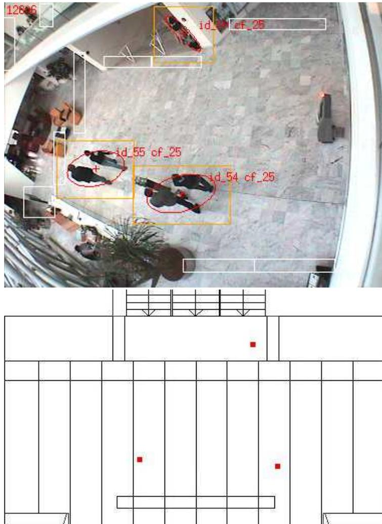
Figure 6.11: Wide-angle camera image of INRIA Rhône-Alpes entrance hall with three targets being tracked (above) and the corresponding target positions on the hall map after applying a homography (below). White rectangles in the camera image (above) indicate the detection zones used by the visual tracker for creating new targets
