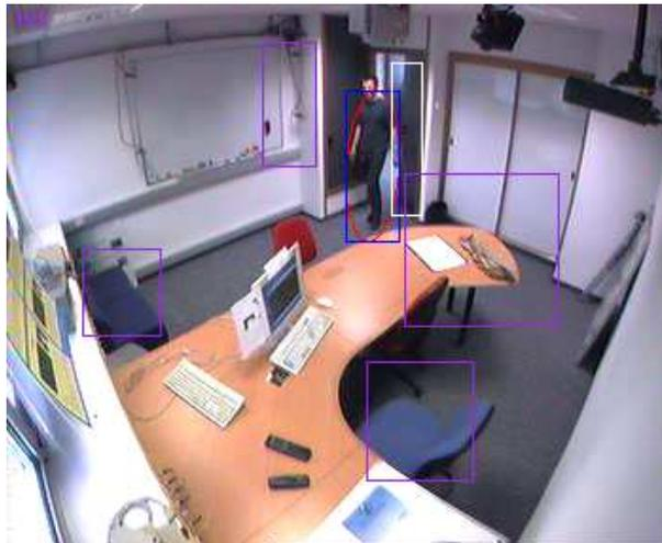
Figure 8.4: Video image of the wide-angle camera of SmartOffice. A white box next to the door is used for the creation of new targets (entities). One person is currently tracked. Four presence detection zones (chair, couch, board and table) of the tracking system are indicated
