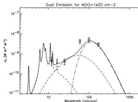
**Fig. 8.** Best fit for the dust infrared emission spectrum, obtained with the Desert et al. model. The brightness corresponds to an interstellar gas column density of  $10^{20} \text{ cm}^{-2}$ . The IRAS and ISOPHOT data are represented by squares. The fit obtained with the model (continuous line) corresponds to the emission of three components: PAHs (dashed line), very small grains (mixed line) and big grains (dot-dot-dot-dashed line).
