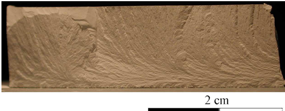
FIGURE II.4.49 – Surface d'une fracture hybride ( \theta = 10^\circ ).
