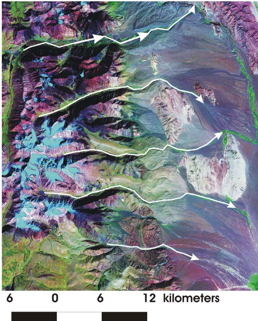
Figure I.9: The right-lateral displacement of rivers due to the Chihtei segment observed on Landsat images. See Figure I.7 for location.
