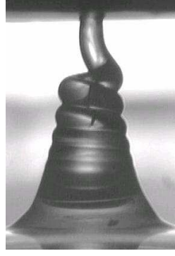
Figure 2.5: Rope of silicon oil with \nu = 1000 \text{ cm}^2/\text{s} , injected from an orifice of radius a_0 = 0.034 \text{ cm} at a volumetric rate Q = 0.0044 \text{ cm}^3/\text{s} and effective fall height H = 0.30 \text{ cm} . is slightly compressed against the plate, so the diameter at bottom is larger than the diameter of the filament near the nuzzle.
