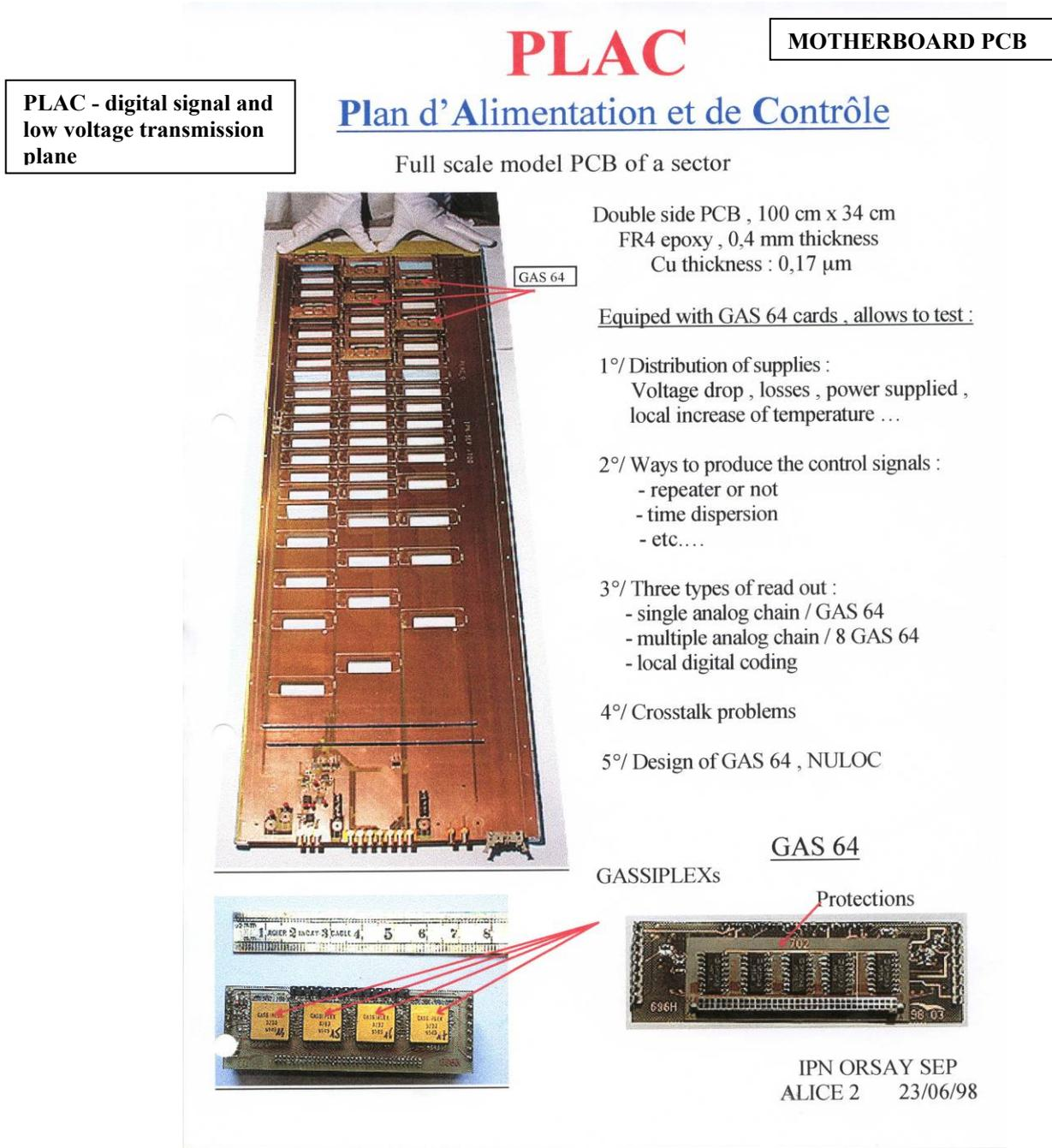
**Figure 67:** View of the first PLAC motherboard (prototype Dec'97) and the GAS64 (prototype Dec'97) daughter boards.
