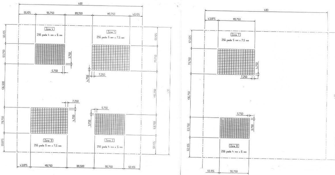
**Figure 83:** Cathode Pad layout for "Plane A" (on the LHS) containing four separate pads regions, labelled zones 1 to 4, and "Plane B" (on the RHS) with two separate pads regions, labelled zones 7 and 8. Plane A has two zones of pads at 4 mm x 6 mm and two at 5 mm x 7.5 mm. Plane B has one zone of with each pad size.
