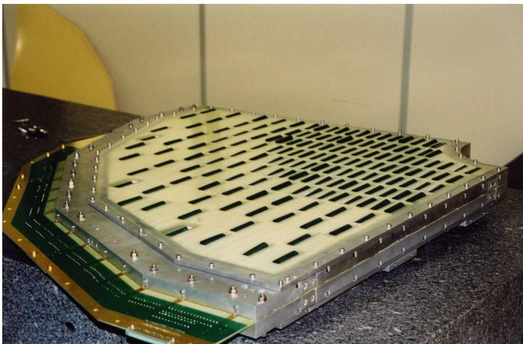
**Figure 64 :** The white Rohacell plane, providing the lightweight mechanical support for the pad plane is seen with the green coloured Kapton foils in folded over in their pigeon holes (to protect them during the mounting process). The anode plane skirt is visible round the outer edge of the detector, extending beyond the aluminium support frames.
