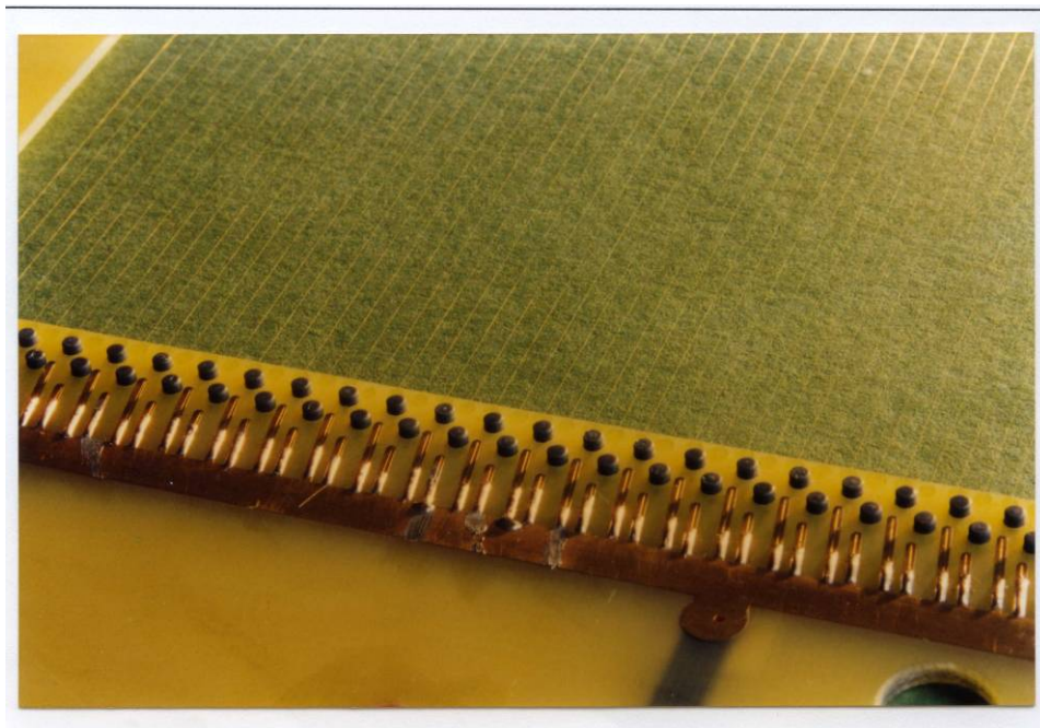
Figure 29 : A photograph of the anode wire plane placed against a dark background to improve the visibility of the 20 \mu\text{m} wires. The black pins are used to align the individual wires, each wire being glued and soldered to the surrounding copper conductor.
