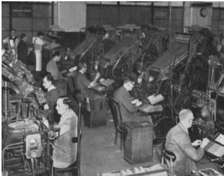
Figure 21 : this is where your paper begins. Operators at work on what Thomas Edison referred to as the “Eighth wonder of the world-Linotypes.” 3
