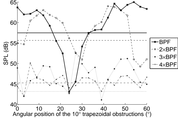
Figure 7.9 Sound pressure level produced by the \Theta = 10^\circ 6-trapezoidal obstruction at optimal axial location z_s^{opt} , measured by the upstream on-axis microphone.
