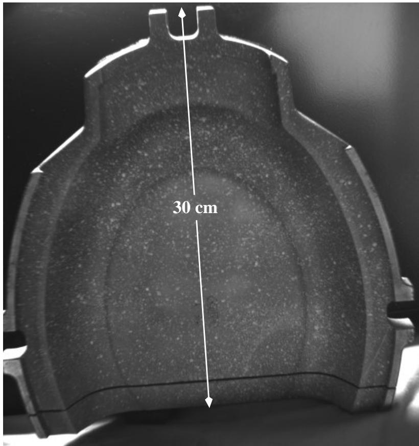
**Fig. 3.21** — *Upper part of a mold used for Pyrex<sup>®</sup> glass plate covered with a spray-painted speckle pattern.*
