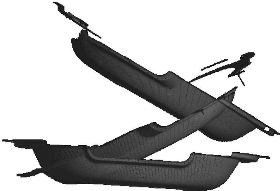
**Fig. 3.27** — *Three clouds of points generated by the 3D scanner, before the registration and fusion. We can notice that the curved parts of the mold are not reconstructed in the two upper clouds.*
