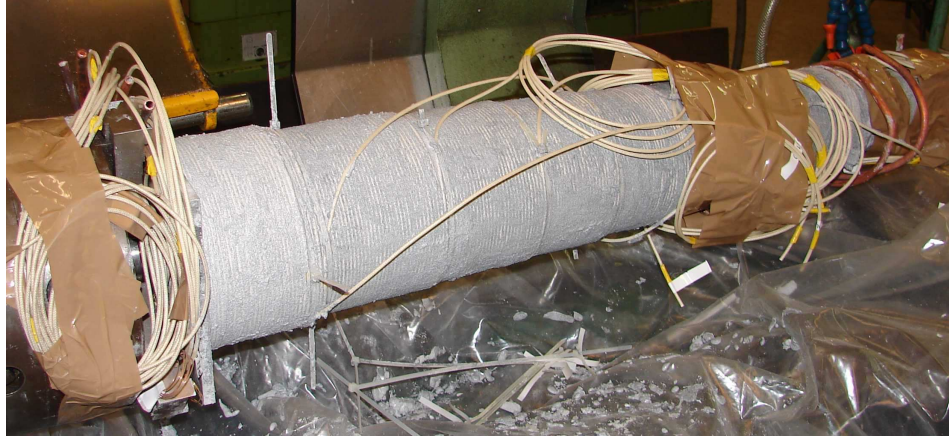
Figure 3.2: The Zeeman slower while being wound. One can see the layer structure of the coils. The cables are held in place using a cement mixed with silicon carbide, which gives a grey color. On the right one can see the end of the two parallel water cooling tubes which are below the coils.
