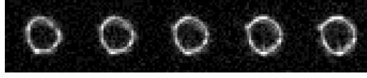
Figure 4.5: Five consecutive ring images distorted by turbulence and detector noise. Each image is 16x16 pixels (13.8''), the average ring radius is 3'', the interval between images is 3 ms, the wind speed is 10 m/s.
