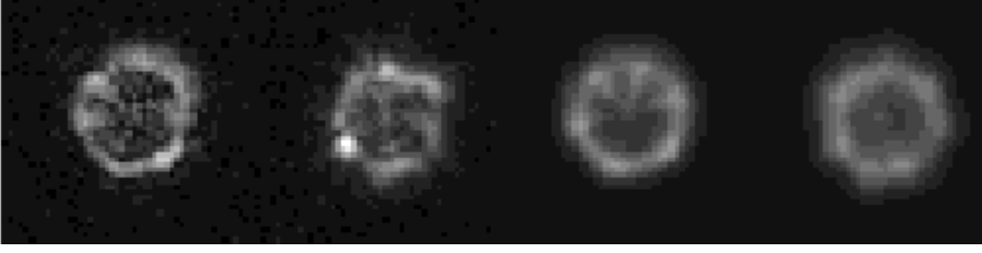
Figure 5.2: From left to right: Simulated ring image – Image of Sirius – Average of 1024 simulated images – Average of 1024 Sirius images. The sequence of Sirius images was recorded on Nov 2 nd at 6:46 UT. The parameters for the data and simulations are given in Sec. 5.8.1.
