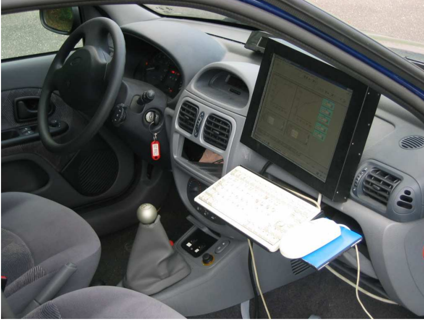
Figure 6.2: View of the cockpit, on the right the screen and the keyboard connected to the IBM computer in the booth can be seen.
