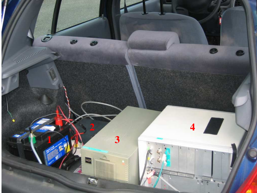
Figure 6.3: View of the rapid prototyping system placed in the booth. 1 Lead-acid battery powering the IBM compatible PC and the interface rack - 2 General switch - 3 IBM compatible PC - 4 interface rack
