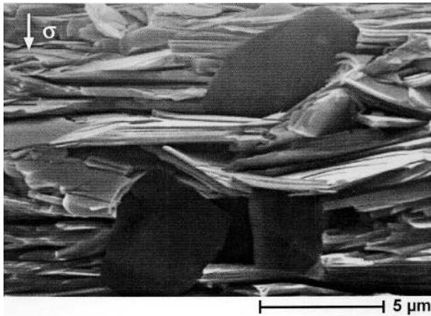
Figure 3. Local misalignment of the 2223 plate-like grains near quasi-isotropic grains of non-superconductive phase.
