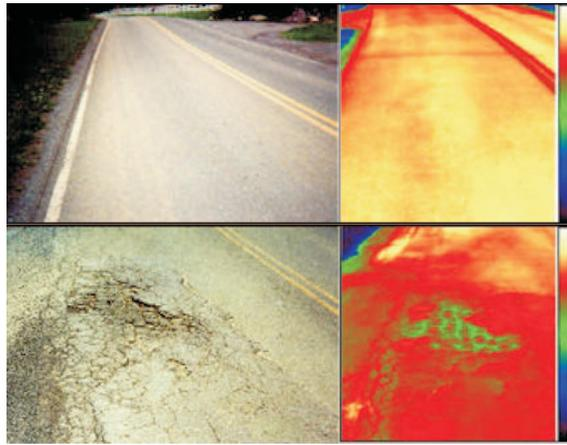
Figure 1.4: Road condition assessment using thermography.
