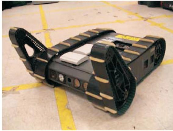
Figure 1.1: Robot used for visual survey at the WTC disaster site.
