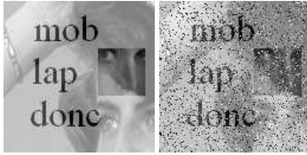
Figure 3.3: Left: clean image; right: noisy image to decompose, it is obtained by adding 20% impulse noise on the left image
