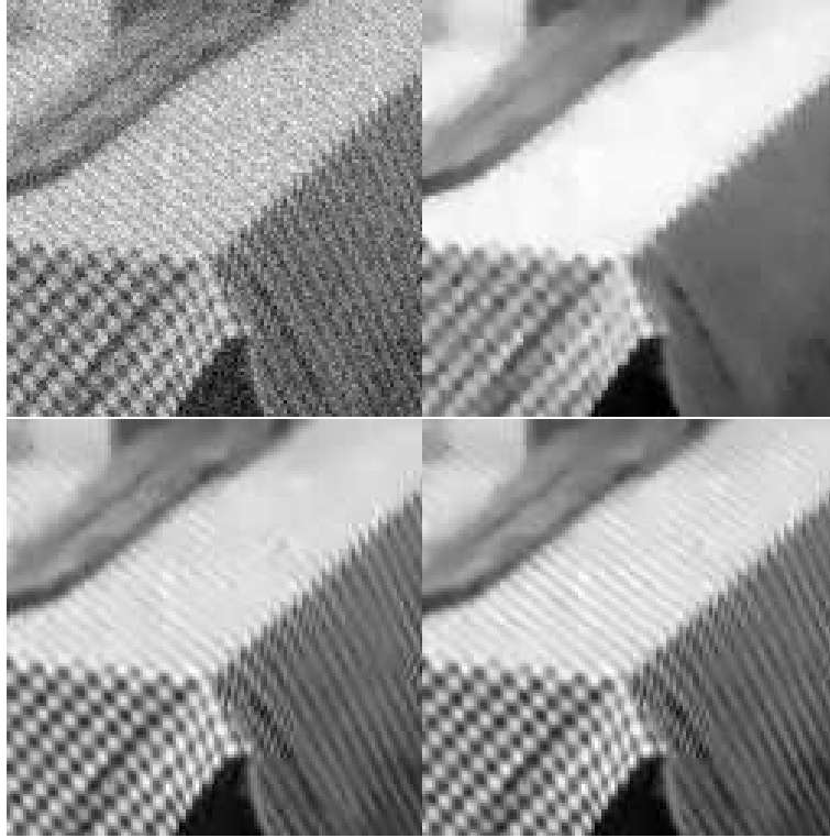
Figure 4.4: Denoising a 128 \times 128 piece of Barbara. From left to right and from top to bottom: noisy image ( \sigma = 20 ), PSNR 22.0896; Rudin-Osher-Fatemi, PSNR 24.2663; K-SVD, PSNR 28.9013; Our new approach, PSNR 29.1148.
