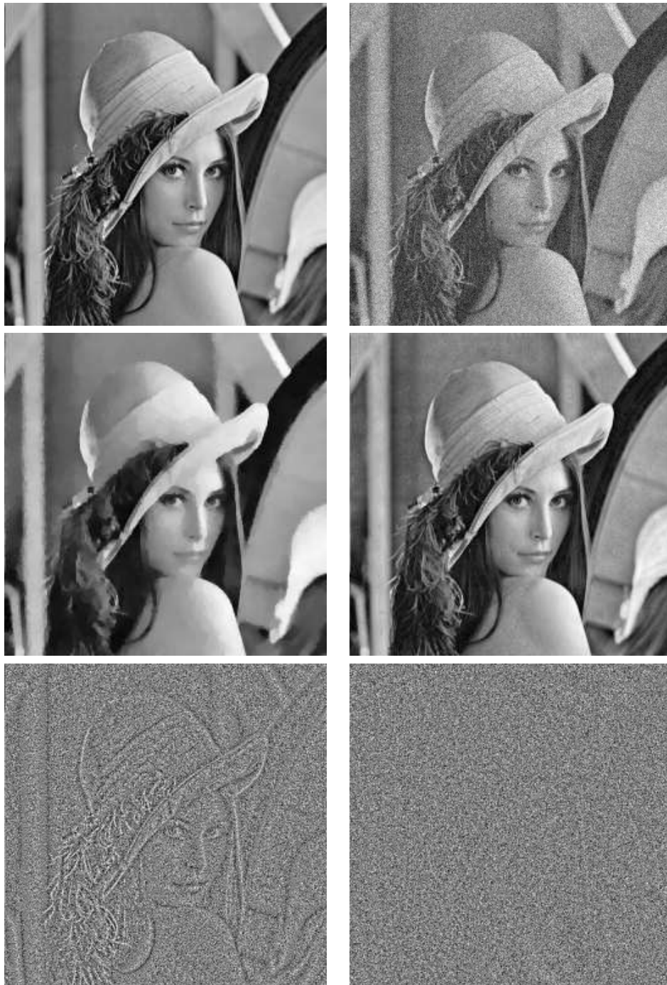
Figure 3.2: Denoising with the ad-hoc dictionary: original image (top-left), noisy image (top-right, \sigma = 20 , PSNR = 22.11); result of the ROF model (middle-left, PSNR = 27.66), result of the general TV - l^\infty with the ad-hoc dictionary (middle-right, PSNR = 34.93); residual of the ROF model (bottom-left), residual of the general TV - l^\infty model (bottom-right)
