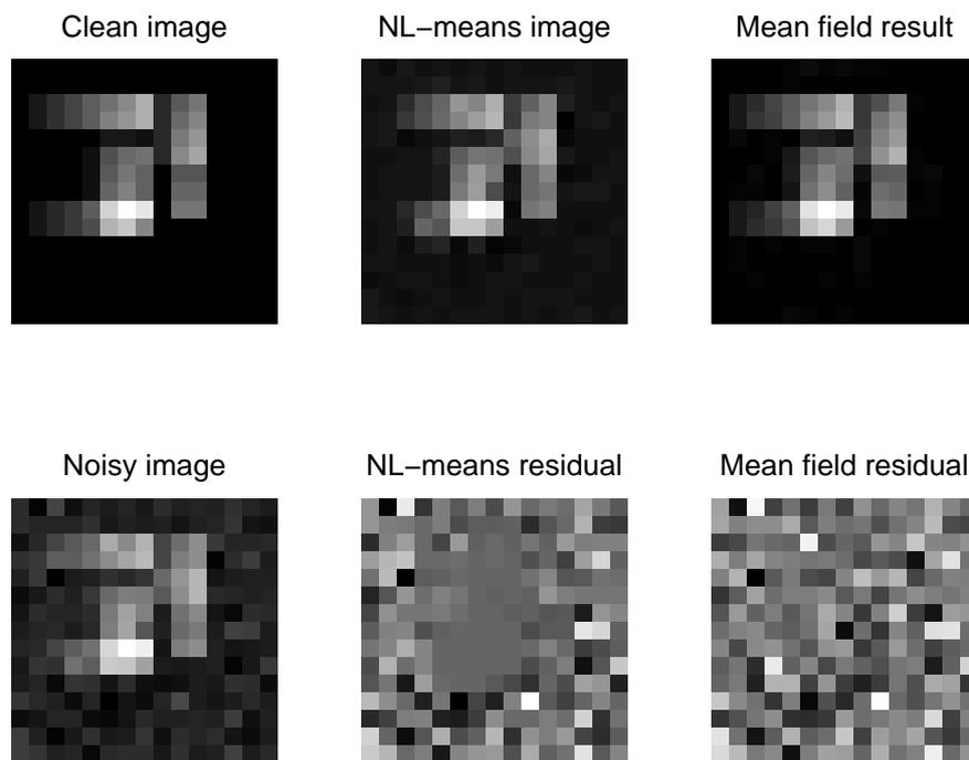
Figure 8.17: Zoom on a zone of Figure 8.16: top-left, clean image; bottom-left, noisy image ( $\sigma = 0.2$ ,  $PSNR = 24.3946$ ); top-middle: NL-means denoising result ( $PSNR = 29.5700$ ); bottom-middle, NL-means denoising residual; top-right: result of mean field approach ( $PSNR = 34.4510$ ), bottom-right: mean field residual
