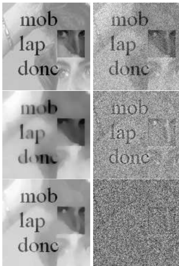
Figure 3.7: Image denoising with known features: top-left: original image, top-right: noisy image with \sigma = 20 , PSNR = 22.0801 ; middle-left: denoise result of the ROF model, PSNR = 24.5559 , middle-right: denoise residual of the ROF model; bottom-left: denoise result of the general TV - l^\infty model, PSNR = 31.1993 , bottom-right: residual of the general TV - l^\infty model.
