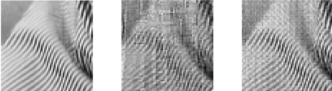
Figure 8.15: Left: original image; MP result(1141 terms) with special DCT dictionary,  $PSNR = 21.4602$ ; reconstruction image of mean field (containing 1141 terms),  $PSNR = 25.7237$ .
