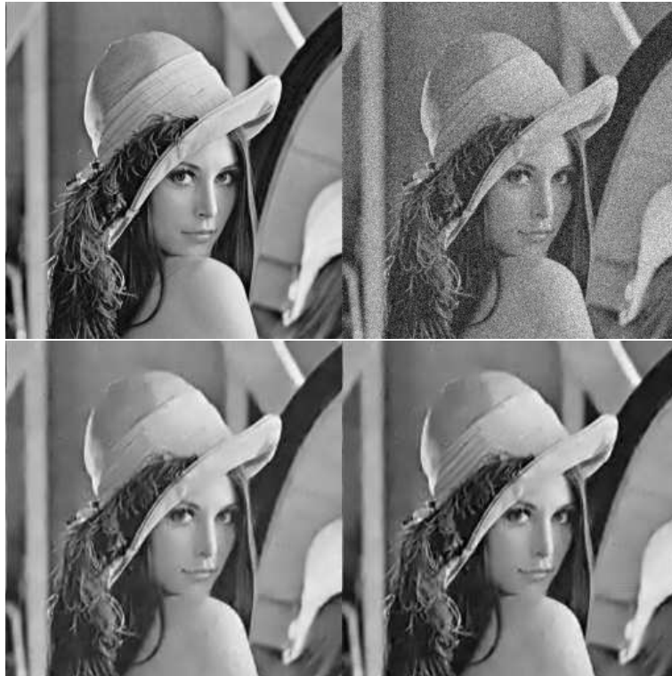
Figure 4.6: Denoising Lenna (size 256 \times 256 ). From left to right and from top to bottom: clean Lenna image, TV 13.8457; noisy image ( \sigma = 20 ), TV 39.9117, PSNR 22.0823; K-SVD result, TV 10.8710, PSNR 30.4464; Our new approach, TV 11.0179, PSNR 30.4688
