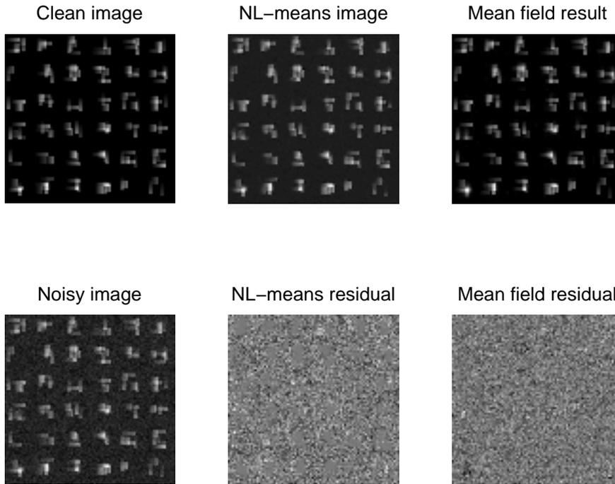
Figure 8.16: Denoising performances: top-left, clean image; bottom-left, noisy image ( $\sigma = 0.2$ ,  $PSNR = 27.5296$ ); top-middle: NL-means denoising result ( $PSNR = 33.6332$ ); bottom-middle, NL-means denoising residual; top-right: result of mean field approach ( $PSNR = 34.7421$ ), bottom-right: mean field residual
