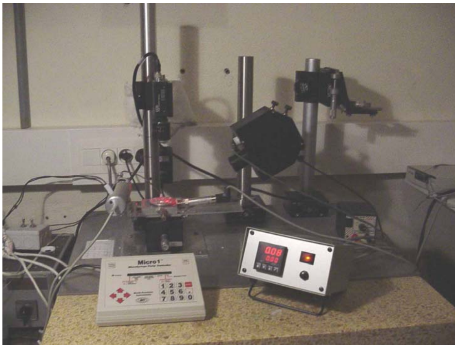
Figure 4-9: Photograph of the complete blister system
