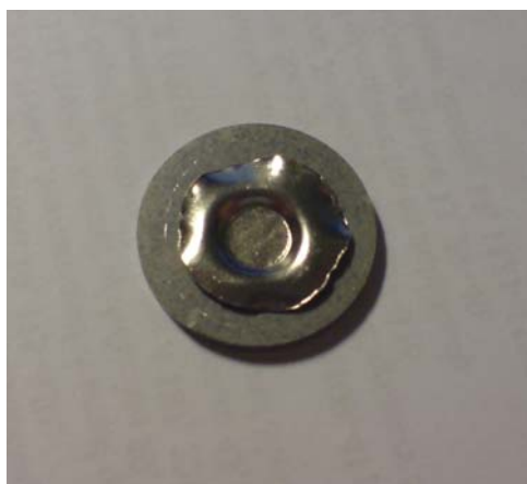
Figure 4-23: After firing, the nickel film separates totally from the substrate.
