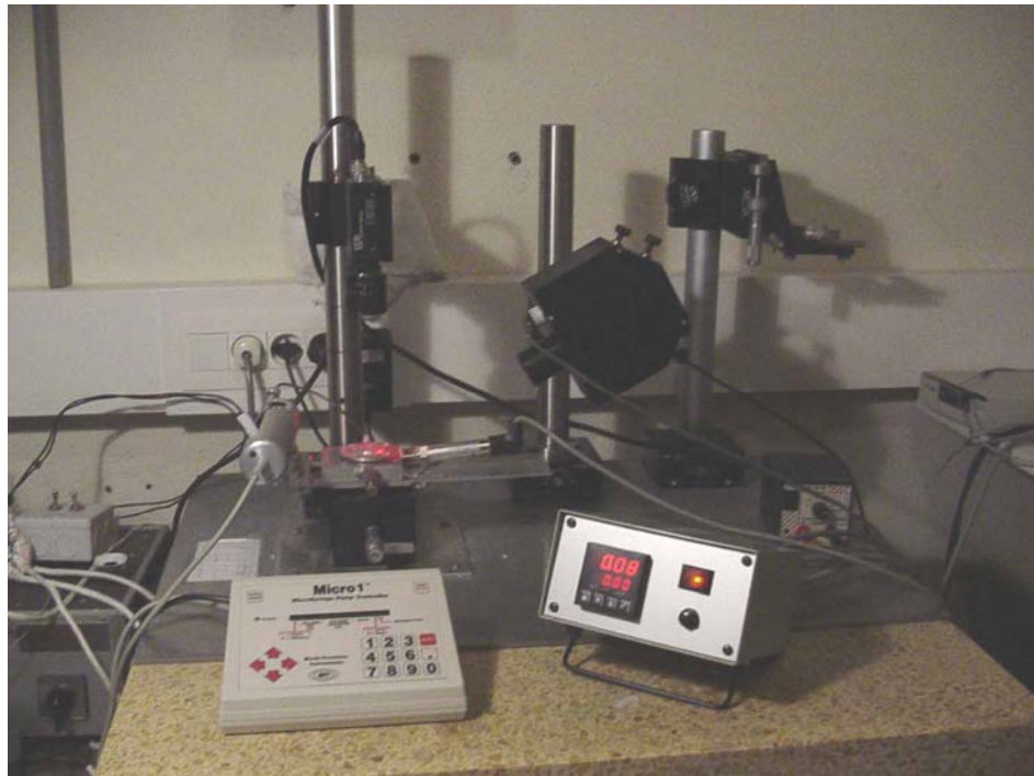
Figure 4-9: Photograph of the complete blister system
