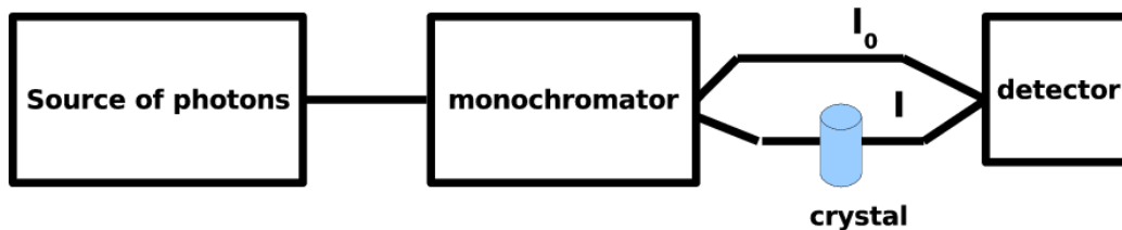
Figure 4.24: Typical setup for absorption tests. The ratio between the intensity of the light crossing the crystal and the intensity of the light having the same optical path through air leads to the absorption coefficient of the crystal
